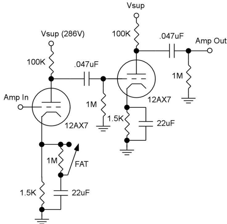
Figure 4-9. Preamp consisting of two triode amplifier stages.
