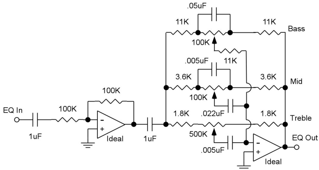
Figure 4-8. Baxandall style equalizer used in Tube Saturator, derived from version by Chu Moy, [http://www.headwize.com/projects/equal\\_prj.htm](http://www.headwize.com/projects/equal_prj.htm).
